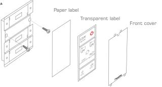
O Insert screws matching the back box into the two mounting holes. Secure the control system to the back box or bracket without overtightening the screws.
