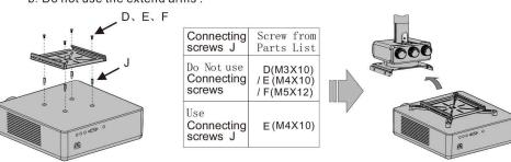
Move the projector mounting plate and adjust the forward/backward slide
