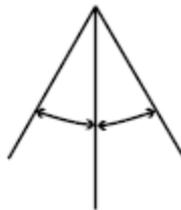
The effective receiving area is about 3 meters with 30° angle from vertical point to the right.
