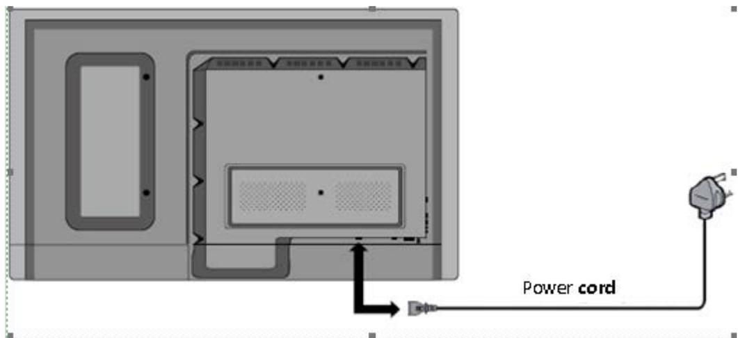
**Step 2** Turn on the rocker switch at the bottom of the interactive panel (next to the power port) to enable power supply. In this case, the indicator is in red.
